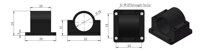
This simple mount acts as combined heat sink mount for 18mm diameter diode modules. Loosen the four small set screws and remove the top half of the module mount to put the laser in. The laser is held firmly by tighten the screws. The module mount reserved 4 through-holes for user to fix the laser on a flat and thermally dissipating surface.
