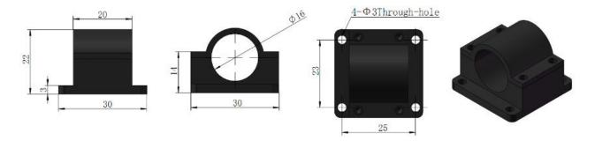
This simple mount acts as combined heat sink, electrical insulator mount for 16mm diameter diode modules. Loosen the four small set screws and remove the top half of the module mount to put the laser in. The laser is held firmly by tighten the screws. The module mount reserved 4 through-holes for user to fix the laser on a flat and thermally dissipating surface.
