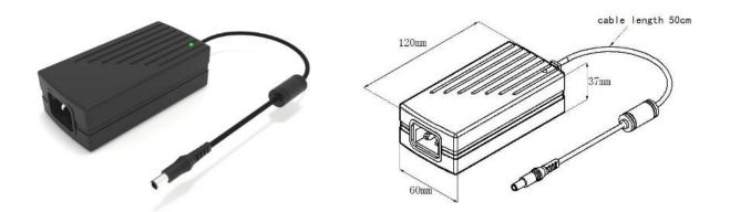
The Universal Diode Laser Module Power Supply with CE-marked provides a well-regulated 5 VDC. This auto ranging power module can be connected to any 85-264 VAC 47/63 Hz supply. There is an IEC 60320 input socket and a 0.5m output cable terminated with an easy connect/disconnect jack socket. The Headset connector which could also be found in accessories is compatible with the power supply jack.
