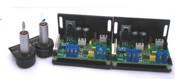
SS2803 is a smart choice if you design a laser projector with a preprogrammed control board inside. It can be tuned up to  $25Kpp@+/-15^{\circ}on$  ILDA 30K test pattern and can do "beam show" as well as "graphic show". SS2803 can display a better details of graphics, such as letters at small scan angle than that of SS2804.
